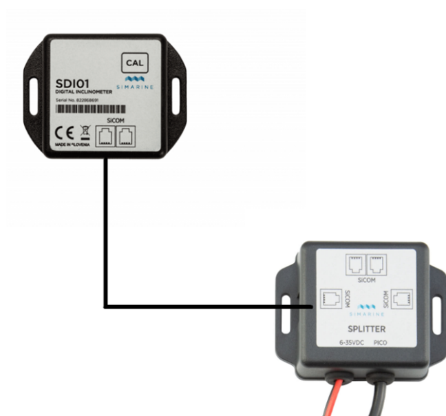
STANDARD WIRING - DIRECTLY TO THE SPLITTER
